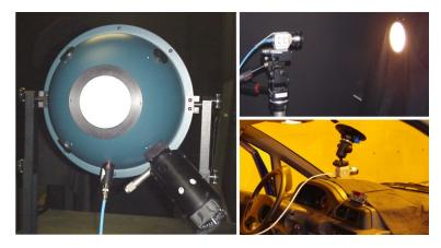
Figure 2 – Integrating sphere of luminance (left), CYCLOPE system during calibration of camera (top right), CYCLOPE system in the vehicle (bottom right)
