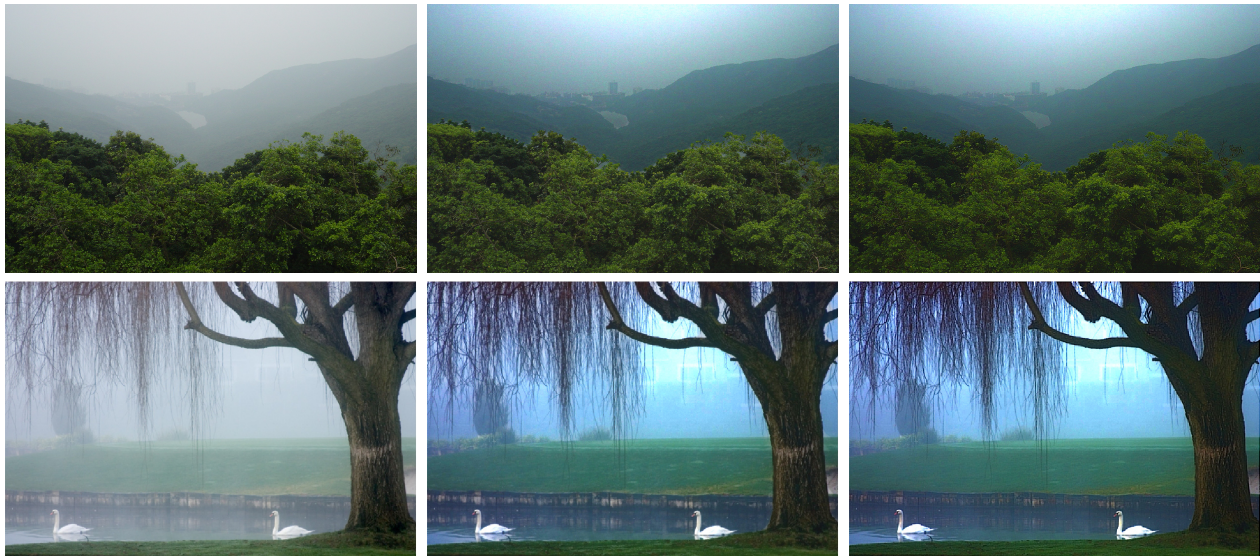
Fig. 11. Example of single image defogging. First column: original foggy images. Second column: fog removal using the fast median filter [21]. Third column: fog removal using the Guided bilateral filter. Notice how halos produced by the median filter are removed with the Guided bilateral filter.
