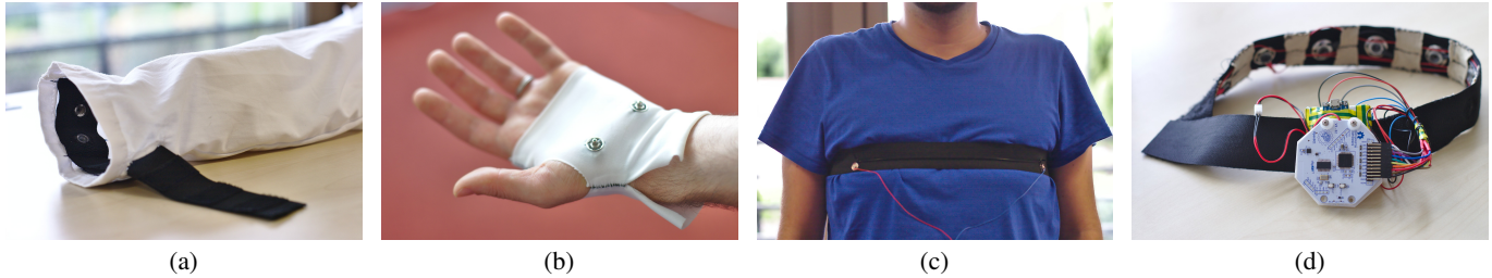
Figure 4: Wearables. a : coat embedding ECG sensors; b : fingerless glove measuring EDA; c : breathing belt; d : EEG headband.
