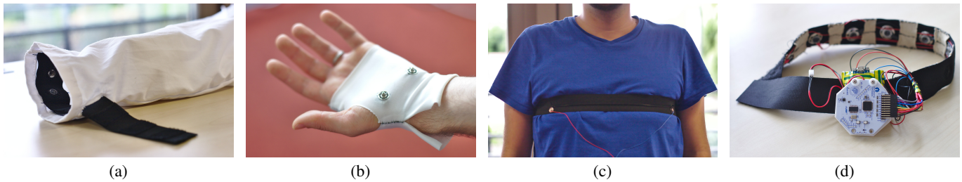
Figure 4: Wearables. a : coat embedding ECG sensors; b : fingerless glove measuring EDA; c : breathing belt; d : EEG headband.
