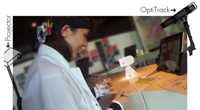
Figure 6: In a scientific museum, various activities were proposed to visitors in order to prompt self-investigation. The setup consists of a projector handling the augmentation and an OptiTrack for the tracking.
