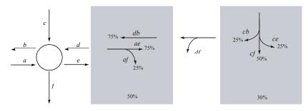
Fig. 5. Diagram of a general intersection and the different phases with the proportion of the green time and turning rates for a given junction
