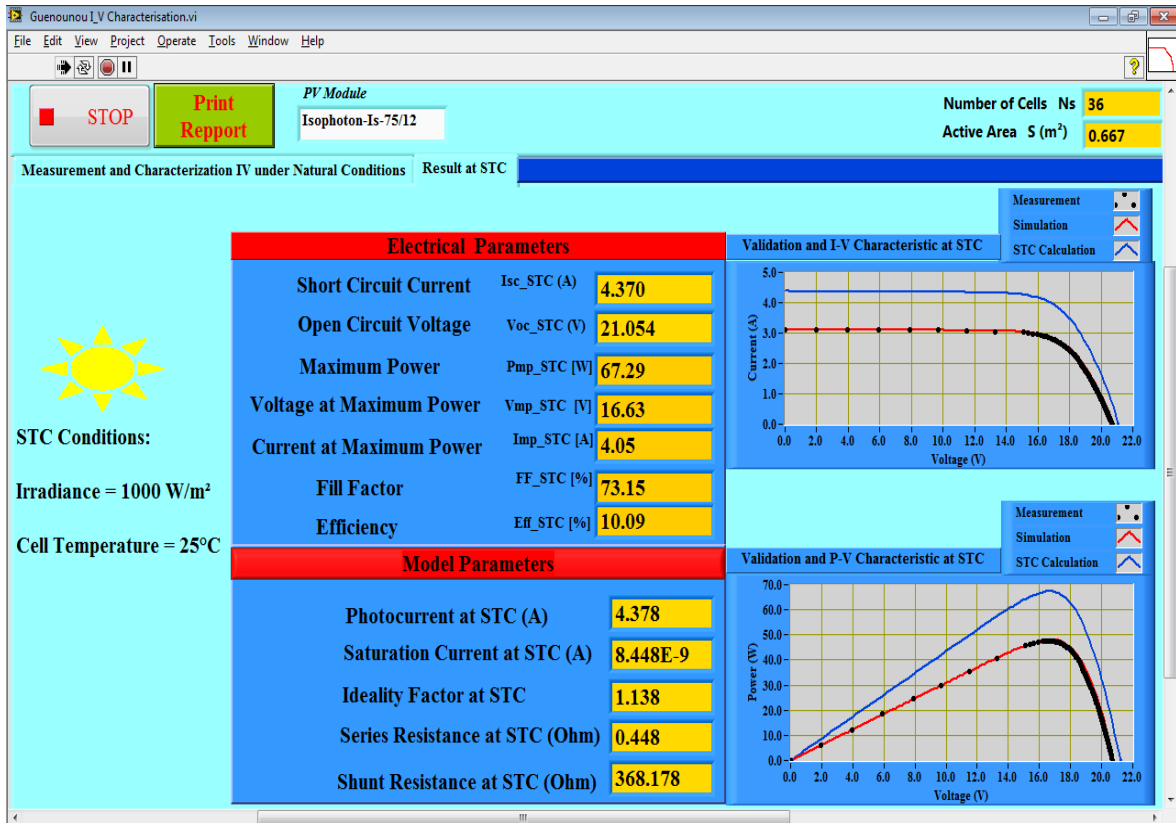
Figure 7. Developed GUI: Validation and STC Results page
