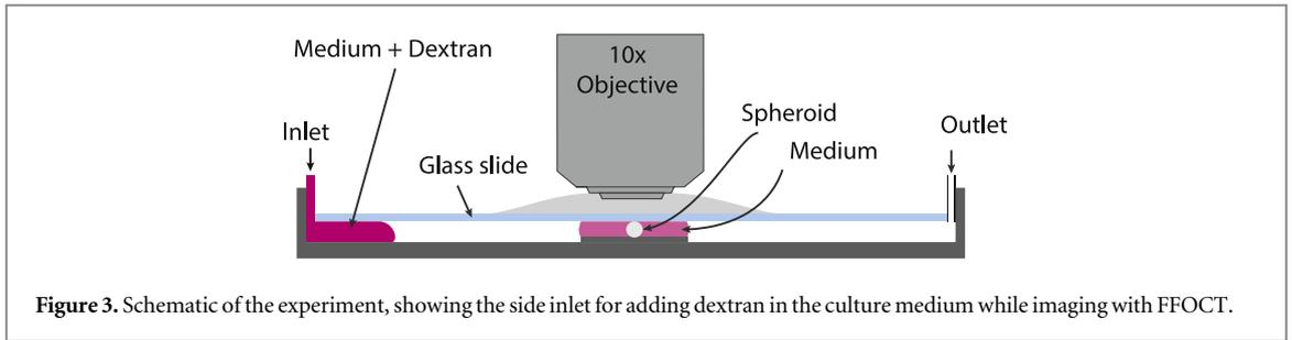
**Figure 3.** Schematic of the experiment, showing the side inlet for adding dextran in the culture medium while imaging with FFOCT.
