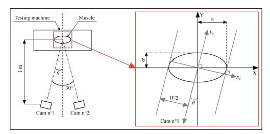
**Figure 2.** Top view of the position of the muscle on the testing machine and of the cameras in front of the muscle (distance and orientation angle  $\theta$ ), and definition of the coordinate systems (XY, and  $x_c y_c$ ), length measured on the picture provided by the camera (W), and the parameters of the ellipsoid (*a* and *b*).
