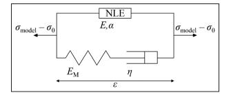
**Figure 4.** Nonlinear viscoelastic model. The nonlinear element is defined with parameters *E* and  $\alpha$ . The Maxwell element is defined with parameters  $E_M$  and  $\eta$ .
