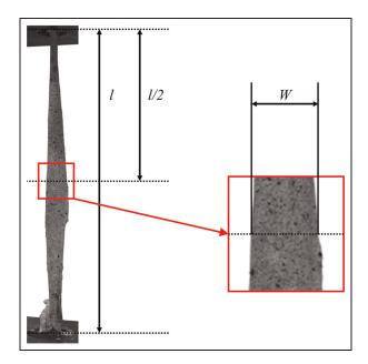
**Figure 3.** Measurements of the different lengths *I* and *W* obtained from the camera images. First, *I* is measured, and then at middle length, *W* is measured in pixels. These measurements are used to define the engineering strain and stress applied to each muscle.
