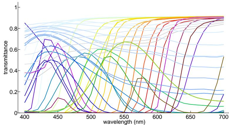
**Fig. 6.** Transmittances of a set of Wratten filters.
