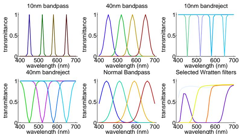
**Fig. 5.** Transmittances of a 4-band filter set.
