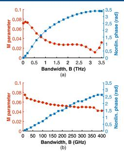
Fig. 4. Misfit parameter to a sinc shape at the output of the laser (red circles) and peak nonlinear phase shift (blue squares) versus filter bandwidth *B* for a flat-top spectral pulse shaper and lasers without (left) and with (right) passive nonlinear propagation in the absence of in-cavity dispersion control.
