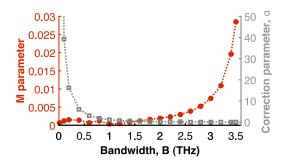
Fig. 5. Misfit parameter to a sinc shape at the output of the laser (red circles) and correction factor  $\alpha$  (gray open squares) versus filter bandwidth B for a Gaussian-top spectral pulse shaper and a laser without passive nonlinear propagation in the absence of in-cavity dispersion control.
