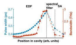
Fig. 3. Evolution of the FWHM temporal (blue circles) and spectral (red triangles) widths of the pulse along the cavity for a flat-top spectral pulse shaper with B=2 THz ( $\tau_p=0.5$  ps). A laser without dispersion control in the cavity is modeled.
