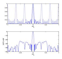
Figure 14: ACF of Costas-LFM signal with  $(t_p \Delta f, t_p B_p) = (3, 17.5)$ , first sidelobe elimination top: continuous  $|R_1(\frac{\tau}{t_p})|$ , dashed  $|R_2(\frac{\tau}{t_p})|$ , bottom:  $|R(\frac{\tau}{t_p})|$
