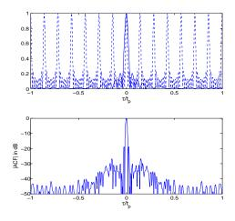
Figure 5: ACF of Costas-LFM signal with  $(t_p\Delta f, t_pB_p) = (7, 24.5), (m, n) = (3, 5)$ top: continuous  $|R_1(\frac{\tau}{t_p})|$ , dashed  $|R_2(\frac{\tau}{t_p})|$ , bottom:  $|R(\frac{\tau}{t_p})|$
