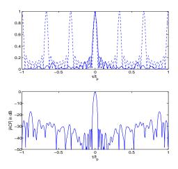
Figure 16: ACF of Costas-Slepian signal with  $(t_p\Delta f, t_pB_p) = (3, 18)$ , first sidelobe elimination top: continuous  $|R_1(\frac{\tau}{t_p})|$ , dashed  $|R_2(\frac{\tau}{t_p})|$ , bottom:  $|R(\frac{\tau}{t_p})|$
