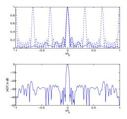
Figure 17: ACF of Doubly coded Costas signal with  $(t_p\Delta f, t_pB_p) = (3, 19)$ , first sidelobe elimination top: continuous  $|R_1(\frac{\tau}{t_p})|$ , dashed  $|R_2(\frac{\tau}{t_p})|$ , bottom:  $|R(\frac{\tau}{t_p})|$
