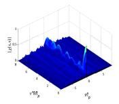
Figure 19: AF of the Costas-P4 signal with  $(t_p\Delta f,t_pB_p)=(3,9)$
