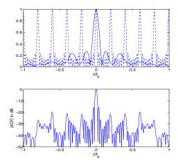
Figure 13: ACF of doubly coded Costas signal with  $(M, N, t_p \Delta f, t_s \Delta f_s) = (8, 4, 5, 0.78)$ top: continuous  $|R_1(\frac{\tau}{t_p})|$ , dashed  $|R_2(\frac{\tau}{t_p})|$ , bottom:  $|R(\frac{\tau}{t_p})|$
