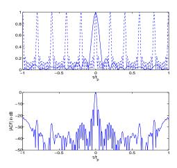
Figure 12: ACF of coded Costas signal using Slepian sequences with  $(t_p\Delta f, t_pB_p) = (5, 10)$ top: continuous  $|R_1(\frac{\tau}{t_p})|$ , dashed  $|R_2(\frac{\tau}{t_p})|$ , bottom:  $|R(\frac{\tau}{t_p})|$
