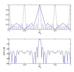
Figure 6: ACF of Phase coded Costas signal using P3 code with  $(t_p\Delta f, L) = (2, 4)$  top: continuous  $|R_1(\frac{\tau}{t_p})|$ , dashed  $|R_2(\frac{\tau}{t_p})|$ , bottom:  $|R(\frac{\tau}{t_p})|$
