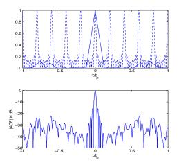
Figure 9: ACF of Phase coded Costas signal using a spectrally balanced Walsh-Hadamard code with  $(t_p \Delta f, L) = (5, 8)$ top: continuous  $|R_1(\frac{\tau}{t_p})|$ , dashed  $|R_2(\frac{\tau}{t_p})|$ , bottom:  $|R(\frac{\tau}{t_p})|$
