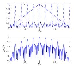
Figure 3: ACF of the Costas code [2,6,3,8,7,5,1,4] in  $|\tau| < t_p$ , for  $t_p \Delta f = 5$  (Grating lobes), top: continuous  $|R_1(\frac{\tau}{t_p})|$ , dashed  $|R_2(\frac{\tau}{t_p})|$  bottom:  $|R(\frac{\tau}{t_p})|$
