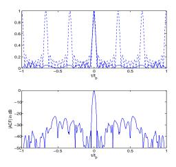
Figure 15: ACF of Costas-P4 signal with  $(t_p\Delta f, L) = (3, 20)$ , first sidelobe elimination top: continuous  $|R_1(\frac{\tau}{t_p})|$ , dashed  $|R_2(\frac{\tau}{t_p})|$ , bottom:  $|R(\frac{\tau}{t_p})|$
