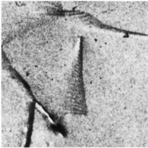
Fig. 6. Traverse topograph, \text{Mo } K\alpha , 220 reflection, Si, 800 \mu\text{m} .
