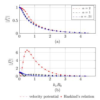
Fig. 3. Dimensionless vertical forces, (a) on buoy (b) on platform, for case study No.2.
