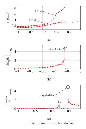
Fig. 2. Matching of the velocity potential (a) and its first derivative (b) and (c) for case study No.3,  $\alpha = .75$ , at the imaginary interface  $r = R_b$  and  $r = R_p$  for  $k_e = 1$ .
