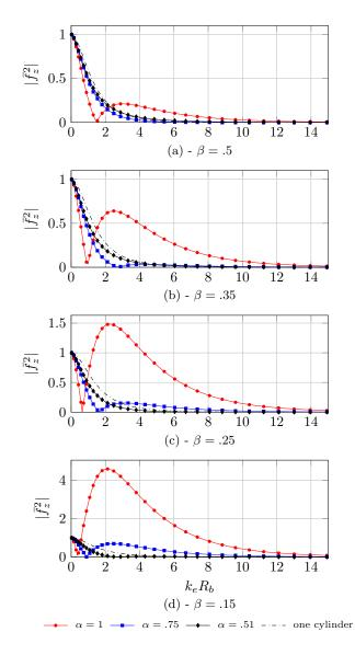
Fig. 12. Dimensionless vertical forces on the platform for differents column and plate radius.
