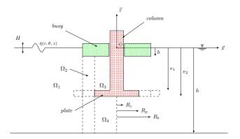
Fig. 1. Definition sketch of the wave energy converter.
