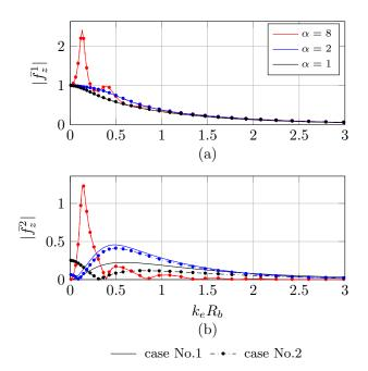
Fig. 4. Dimensionless vertical forces, (a) on buoy (b) on platform.
