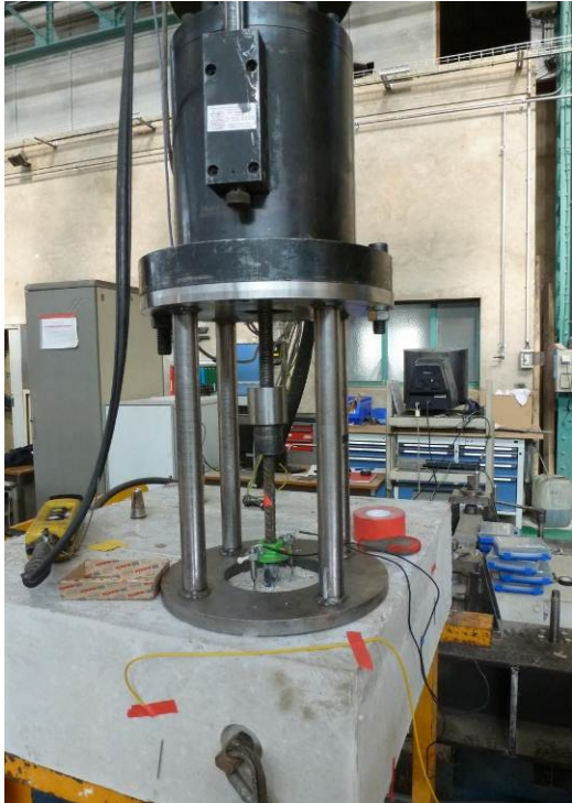
Figure 9. Principle of the direct tension pullout bond test and overall view.
