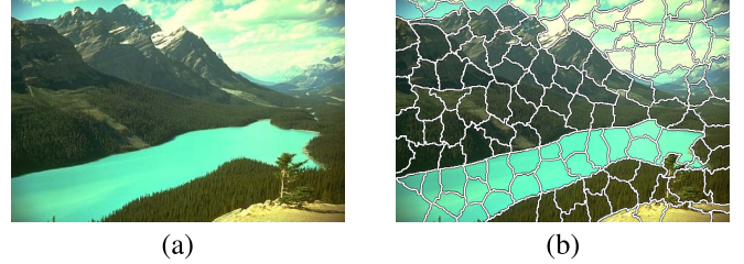
Fig. 1. Superpixels illustration. The original image comes from the Berkeley segmentation database. (a) Original image. (b) Waterpixels.
