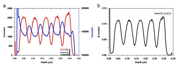
Fig. 2. (a) SIMS elemental concentration depth profiles of B and Al for the sample grown on GaN template, (b) Boron content in solid layers calculated from SIMS by using boron implanted AlN sample as reference.
