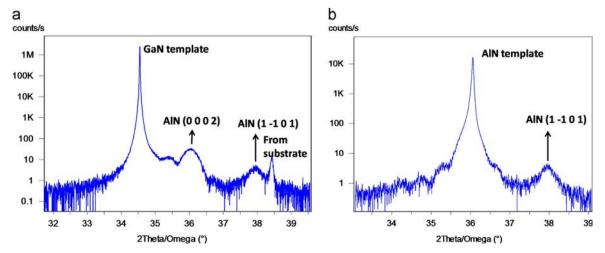
**Fig. 4.** h-XRD  $2\theta$ - $\omega$  scans of 5-period AlN/BAlN heterostructure grown on (a) GaN template and (b) AlN template.
