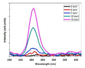
**Fig. 6.** Cathodoluminescence spectra at 77 K of 5-period AlN/BAIN heterostructure grown on AlN template.
