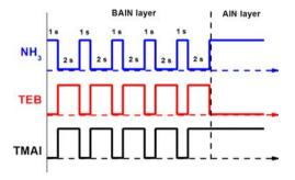
Fig. 1. Schematic of precursors feeding sequence for BAIN and AIN.
