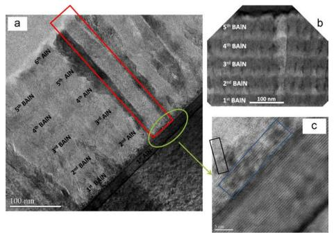
**Fig. 3.** (a) STEM images (bright-field) of 5-period AlN/BAIN heterostructure grown on AlN template and columns are clearly observed in the structure; (b) HAADF–STEM image to show better contrast of BAIN and AlN layers; and (c) high magnification of the zone where the 1<sup>st</sup> BAIN layer starts to grow.
