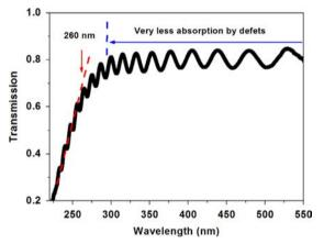
**Fig. 7.** Transmission spectrum at room temperature of 5-period AlN/BAIN heterostructure grown on AlN template.
