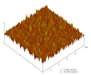
$\begin{tabular}{ll} {\bf Fig. 5.} & Atomic force microscopy (AFM) image of 5-period AlN/BAIN heterostructure (310 nm for total thickness). \end{tabular}$
