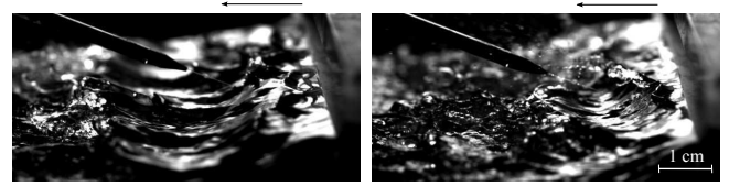
FIG. 7. Impact of forcing on the wavelength of the shear instability for U_G = 27 m/s and U_L = 0.28 m/s; Left: no forcing; Right: forcing with pulsed jet at 34 Hz, midchannel u_{rms}/U_G = 0.09 . The forcing leads to a decrease in the wavelength.
