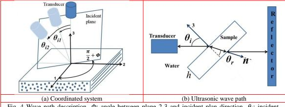
Fig. 4 Wave path description.  $\Phi$ : angle between plane 2-3 and incident plan direction.  $\theta_i$ : incident angle.  $\theta_r$ : refraction angle
