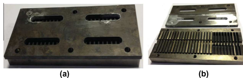
Fig. 2. Designed high temperature titanium tool for the reflow operations. (a) Assembled and (b) decomposed.
