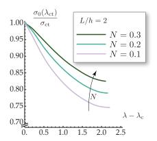
Figure 9: Ratio of the effective true stress to the average true stress as a function of the additional stretch after bifurcation at the center of the neck as predicted by the one-dimensional model of the block for three values of the strain hardening exponent. The effective true stress is the stress which would occur at the stretch  $\lambda$  if the block were constrained to deform uniformly.
