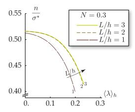
Figure 7: Normalized load  $n/\sigma^*$  versus the additional average stretch after bifurcation in the region  $0 \le X \le h$ ,  $\langle \lambda \rangle_h \equiv x(h)/h - \lambda_c$ . The block material is elastic-plastic with N=0.3 and  $\sigma^*/E=0.003$ . As seen above, this relation is essentially independent of the initial aspect ratio if  $L/h \ge 2$ , and these curves are virtually unchanged when  $\sigma^*/E$  is increased from  $10^{-3}$  to  $10^{-2}$ .
