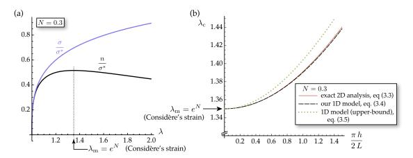
Figure 2: (a) The true stress  $\sigma$  and the nominal stress n for the power law material defined by equation (3.6) with N=0.3. (b) An example comparing the stretch at bifurcation for a block of thickness h and half-length L in the undeformed state, as derived from the exact two-dimensional analysis (3.3) by Hill and Hutchinson (1975), from the one-dimensional model (3.4) derived in this paper, and from the approximate one-dimensional model (3.5) of Coleman and Newman (1988).
