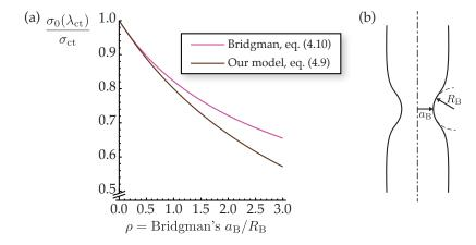
Figure 10: (a) Comparison between Bridgman's 'correction factor' and the result from the one-dimensional reduction for a round bar, expressed in terms of the ratio  $\rho$  of the cross-sectional radius to the radius of curvature at the center of neck. (b) Using Bridgman's notation,  $\rho = a_{\rm B}/R_{\rm B}$ .
