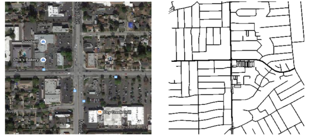
Fig. 3. San Jose (California) urban area captured from Google Maps (left) and exported to a VANET network topology by using MOVE/SUMO (right)
