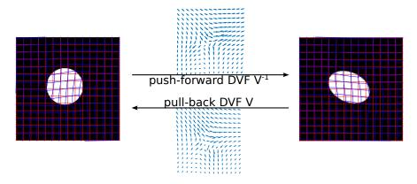
Figure 3: warping between grids; The pull-back DVF provides the mapping back to initial grid of the circle. The inverse,  $V^{-1}$ , serves to reconstruct values from the circle's grid onto the ellipse's grid. Deformed indexing grids are shown in blue. Arrows indicate the direction of registration.
