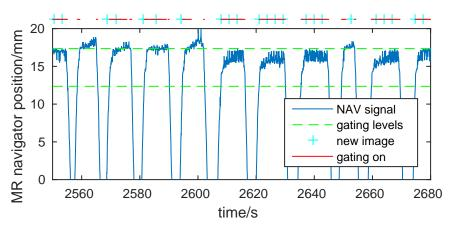
Figure 4: Navigator data with acceptance window: between the gating levels, imaging and beam generation becomes active. While the MR volumes are sampled, the plan segments are gradually delivered according to the treatment plan and the gating intervals. The high gating efficiency ( $\approx 53\%$ ) is clearly recognizable.
