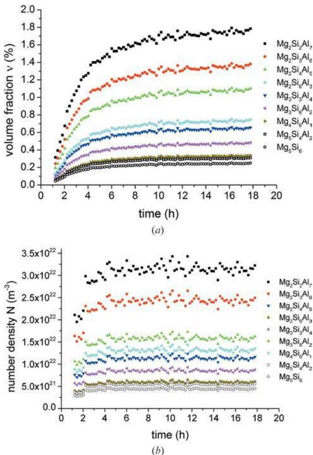
**Figure 5** Precipitate volume fraction (a) and number density (b) for experiment AA calculated from SANS data using different precipitate compositions. Filled symbols: compositions of pre-stages of  $\beta''$  precipitates supposed to be occurring sequentially during ageing (Chen *et al.*, 2006). Open symbols: compositions suggested for fully evolved  $\beta''$  precipitates (Hasting *et al.*, 2009; Zandbergen *et al.*, 1997)
