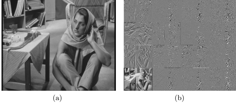
Figure 2. First level of Polynomial Transform with a 4 \times 4 Hermite complete basis.
