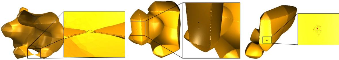
Fig. 11. DELISO mismatch example. From left to right: holes in  $C^0$  regions; single missing triangle in a smooth region; duplicated vertex (the mesh around the duplicated vertex is shown). These behavior induce topology mismatches between the generated mesh and the expected topology.
