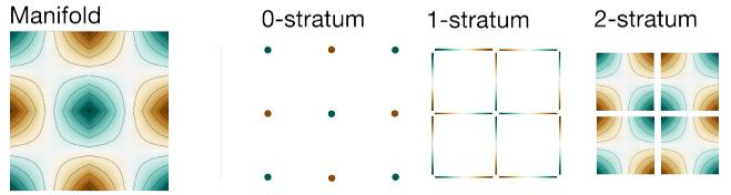
Fig. 6. An illustration of a piecewise-smooth immersed manifold. The colormap illustrates the value of each point of the scalar field. Notice that although the manifold itself is not everywhere differentiable, each stratum is itself an open manifold that is differentiable.
