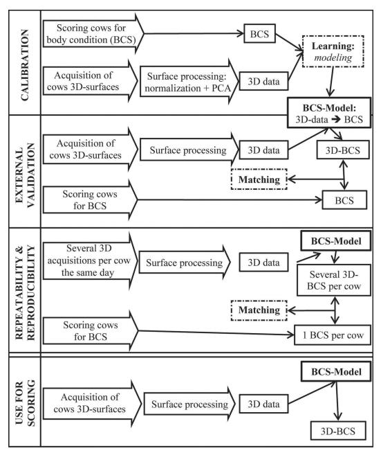
Figure 1. Methodology to estimate BCS with 3-dimensional surfaces: calibration, external validation, repeatability, and reproducibility and use for scoring.
