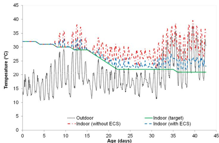
**Figure 2.** Comparison of predicted indoor temperatures in two broiler houses using or not an evaporative cooling system (ECS), during a heat wave in Western France in 2003.
