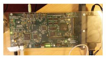
**Fig. 1**: Texas Instruments TMS320C6713 floating point digital signal processing platform.
