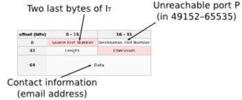
Fig. 2. UDP PING: UDP Packet structure
