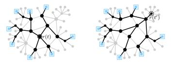
Fig. 2. Left: a set of monitors (the squared nodes) send probes towards a target IP address t and obtain the four interfaces of router r(t). Right: the same monitors send probes towards another target t' but miss most interfaces of r(t').
