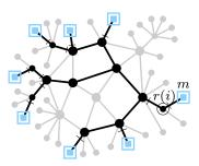
Fig. 5. If we target an interface i that belongs to a border router r(i) then our measurements may see more than one interface for r(i). However, only one of them does not belong to B(M), as displayed in this picture: all interfaces of B(M) are marked with a small dash.
