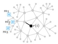
Fig. 4. Three monitors,  $m_1$ ,  $m_2$  and  $m_3$  are actually colocated, and therefore they may observe a unique interface for any given target router r(i). They are redundant regarding the quality of the measurement.
