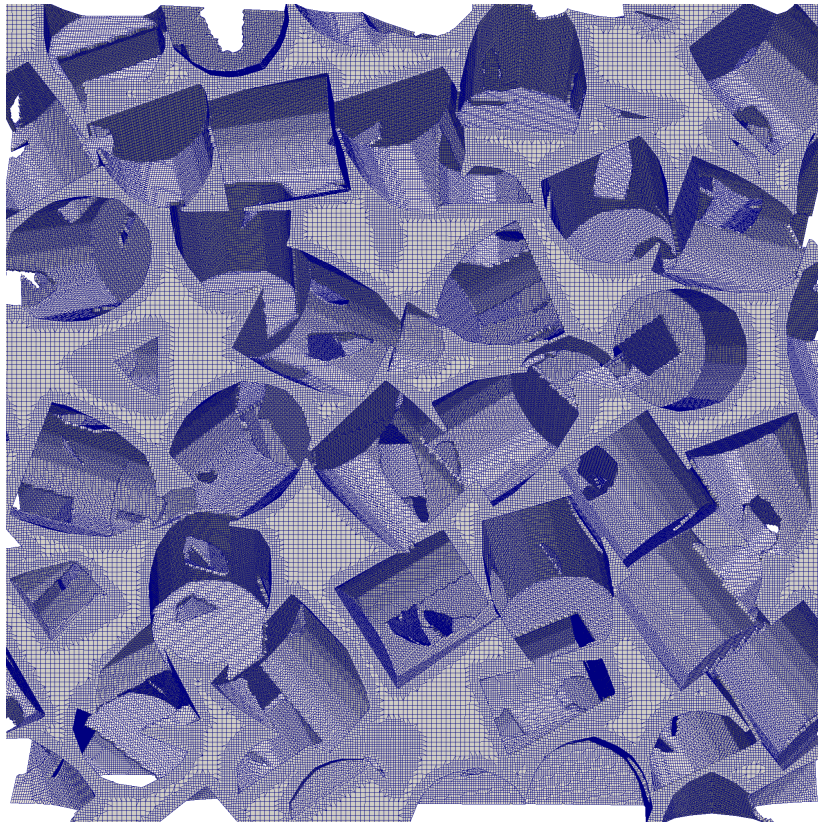
Figure 3: View of the final mesh, packing of cylindrical beads.
