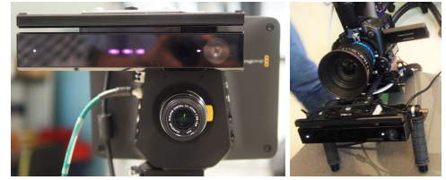
Fig. 2. Our system using different film cameras coupled with the Kinect 2. Left: Blackmagic Studio HD with 14mm lens. Right: Panasonic AG-AF100A with a 18mm lens.
