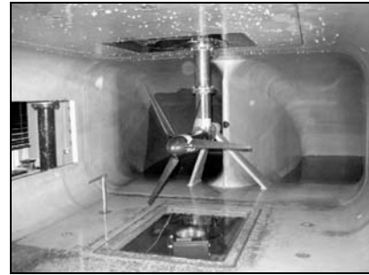
Fig. 6. The tested marine turbine [27].
