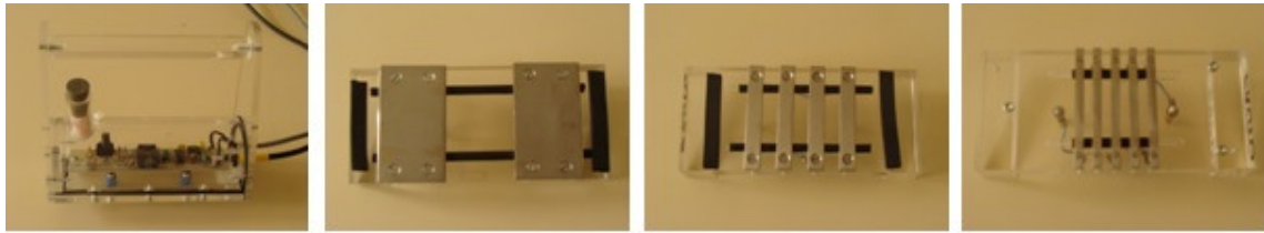
Figure 7. Photos of the capacitive probe system and of the three different associated electrodes
