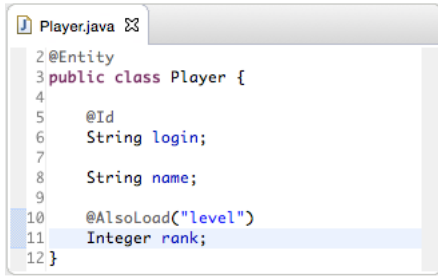
Fig. 3: Lazily migrating legacy entities: A developer has renamed attribute level to rank . Annotation @AlsoLoad ensures that a legacy attribute level can still be loaded and will be renamed to rank .
