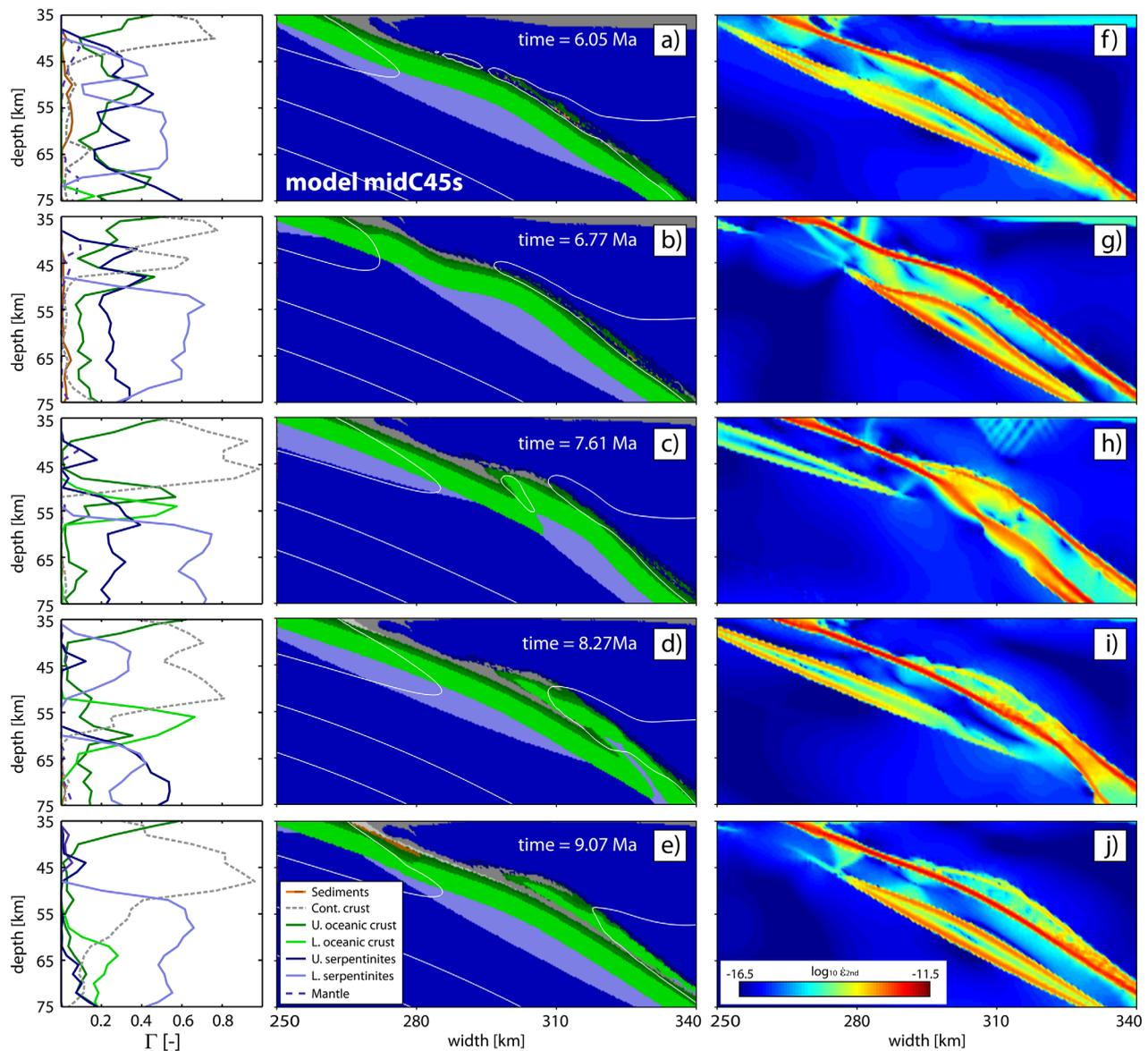
**Figure 6.** (a–e) Snapshots of marker distribution of the discontinuous reference model between 6 and 9 Myr. (f–j) According plots of the second invariant of the strain rate tensor. Left column: Percentages of rock type involved in the main subduction shear zone versus depth (markers with strain rates larger than  $10^{-13} \text{ s}^{-1}$ ).
