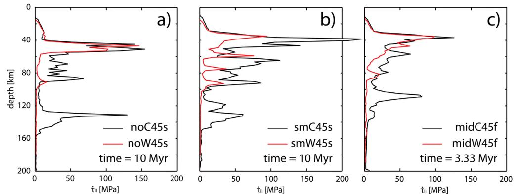
**Figure 11.** Second invariant of the stress tensor along the subduction interface. (a) Experiments without oceanic plate serpentinization. (b) Experiments with small patches. (c) Experiments with fast convergence. Black lines: “cold” models. Red lines: “warm” models.
