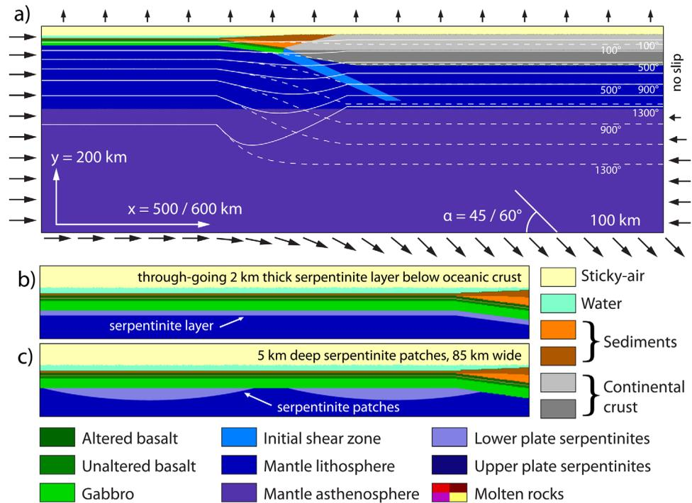
**Figure 2.** Model setup. (a) Complete model size. Colors define initial rock marker type. White lines illustrate initial temperature distribution (Full line: “warm” continent; Dashed line: “cold” continent). Arrows: lateral velocity boundary conditions, (b) initial distribution of continuous oceanic mantle serpentinization. (c) Initial distribution of discontinuous distribution with medium-sized patches (85 km).
