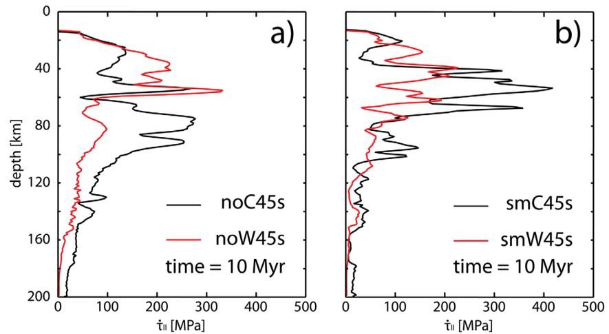
**Figure 7.** Averaged values of the second invariant of the stress tensor within lower oceanic crust (gabbro) of experiments without slicing: (a) “cold” (black) and “warm” (red) models without oceanic mantle serpentinization. (b) “Cold” (black) and “warm” (red) models with small patches of discontinuous oceanic mantle serpentinization (42.5 km).
