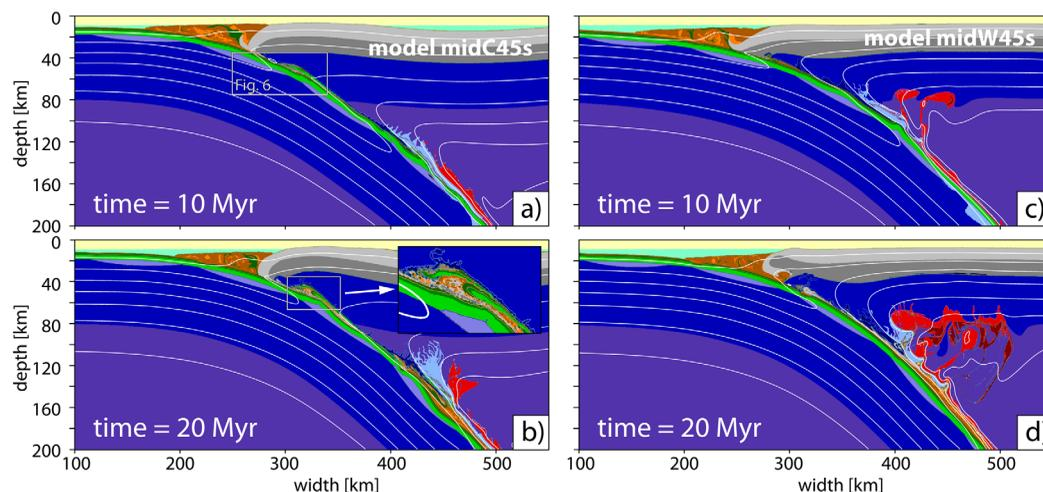
**Figure 5.** Snapshots of the reference model for experiments with discontinuous slab serpentinization after  $\sim 10$  Myr and  $\sim 20$  Myr for (a, b) “cold” and (c, d) “warm” continental geotherms.
