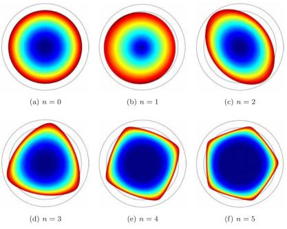
Fig. 4. The modal shapes of Brain in the case of rigid skull: the colors pertain to the Von Mises stress.
