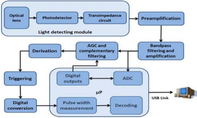
Figure 4: Synopsis of the VLC receiver.
