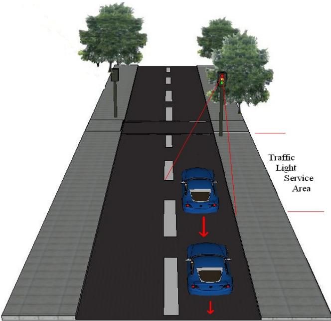
Figure 1: Illustration of the proposed scenario: the traffic light sends a message that is received by the first car and retransmitted to the car behind.
