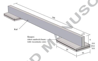
Fig. 6. Rail on sleepers modeled by short sandwich beams with viscoelastic core.
