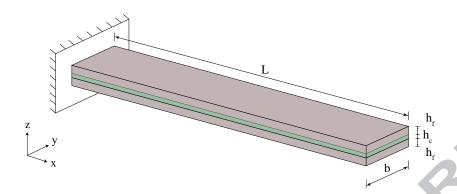
Fig. 1. Sandwich beam structure.
