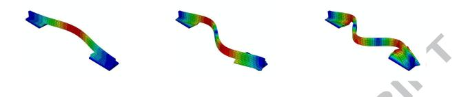
Fig. 7. First three modes for the model of rail on sleepers.
