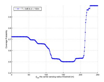
Fig. 4. The coverage probability vs  $d_{CS}$ , the radius of carrier sensing domain for d = 150m, radius of the coordinated set and for different values of the SINR threshold
