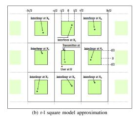
Fig. 1. Stadium dense WLANs: approximation using r - l square Point Process
