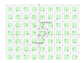
Fig. 2. The r-l square p.p., the serving AP is the nearest one to the typical user, APs inside the CS domain are silenced by the CSMA/CA procedure and APs in  $(\mathcal{A})$  are APs inside the coordinated set and outside the carrier sensing domain
