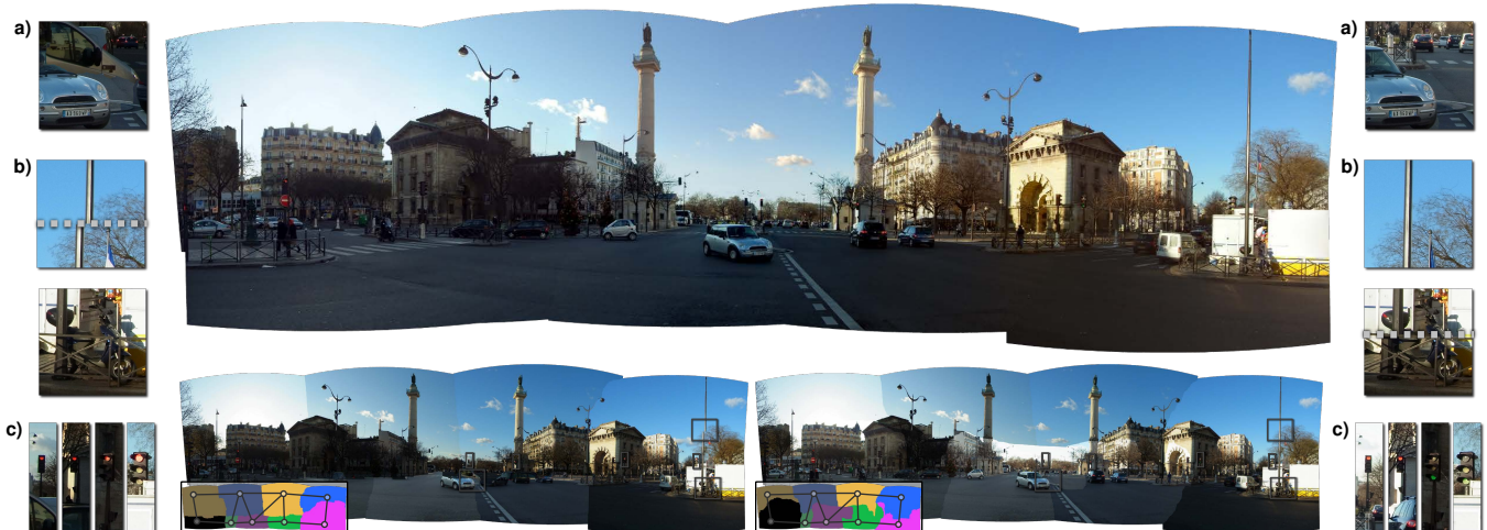
Figure 1: Panorama Weaving on a challenging data-set (Nation, 12848 x 3821, 9 images) with moving objects during acquisition, registration issues and varying exposure. Our initial automatic solution (bottom, left) was computed in 4.6 seconds at full resolution for a result with lower seam energy than Graph Cuts. Additionally, we present a system for the interactive user exploration of the seam solution space (bottom, right), easily enabling: (a) the resolution of moving objects, (b) the hiding of registration artifacts (split pole) in low contrast areas (scooter) or (c) the fix of semantic notions for which automatic decisions can be unsatisfactory (stoplight colors are inconsistent after the automatic solve). The user editing session took only a few minutes. (top) the final, color-corrected panorama.
