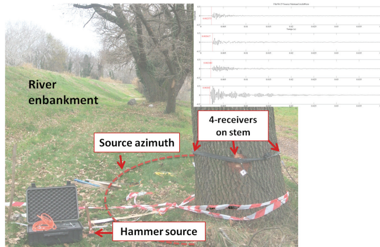
Fig. 5. Example of in-situ experiment using RINNTECH® methodology on Rhône river embankment
