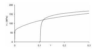
**FIGURE 7.** Simulation results for the stress-strain behaviour of an IF steel during monotonic and cross test.
