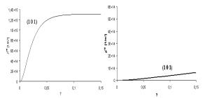
**FIGURE 3.** Evolution of the intensity and polarity of the dislocation walls in a crystal with initial orientation (-27.2°, 133.4°, 53°) during a shear test.
