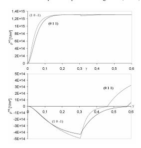
**FIGURE 4.** Evolution of the intensity and polarity of the dislocation walls in a crystal with initial orientation (43.3°, 127.2°, -43.2°) during a reverse test.
