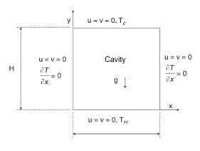
y = 0 whereas a low dimensionless temperature  $\theta(x, y = 1) = \theta_C = -0.5$  is applied on the upper boundary. The dimensionless temperature  $\theta$  is defined by:
