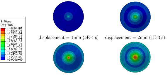
displacement = 3mm (1.5E-3 s) displacement = 4mm (2E-3 s)
