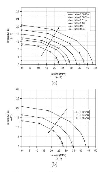
Figure 4: Strain rate (a) and temperature (b) influence on stress evolution for tension-shear loading numerical tests.
