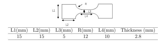
Figure 1: Specimens dimensions.
