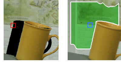
Figure 3: Illustration of the proposed depth-aware search. Left: Hole to inpaint (in black), with the target patch depicted in red. Right: search space in the original view (in green), with the best patch depicted in blue. One can notice that the cup (foreground) does not belong to the search space which is restricted to the background.
