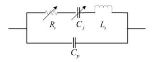
Fig. 2. Equivalent model of the varactor diode.
