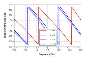
Fig. 13. Phase shifting for different values of the capacitance.
