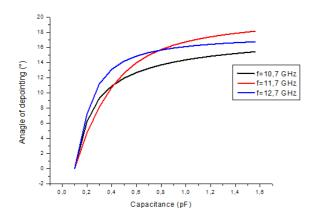
Fig. 15. Depointing versus capacitance for different frequencies of network depointing.
