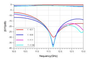
Fig. 7. Return and insertion losses with varactor diode for different values of the capacitance.
