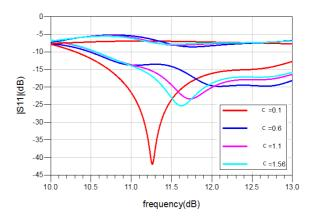
Fig. 12. Return and insertion losses for different capacitance values.
