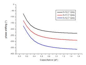
Fig. 9. Phase shift versus capacitance for different frequencies of the proposed phase shifter.
