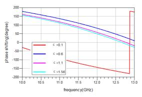
Fig. 8. Phase shifting with varactor diode for different values of the capacitance.
