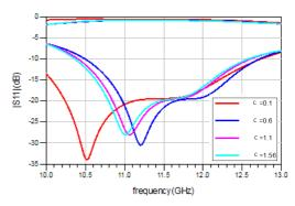
Fig. 4. Return and insertion losses for different values of the capacitance.
