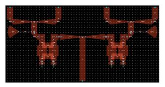
Fig. 11. Electronically steerable beam antenna array with varactor diode.
