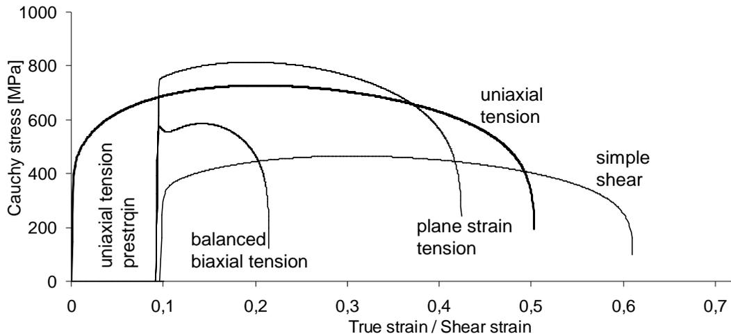
**FIGURE 7.** Different loading paths simulations after a uniaxial tensile prestrain.
