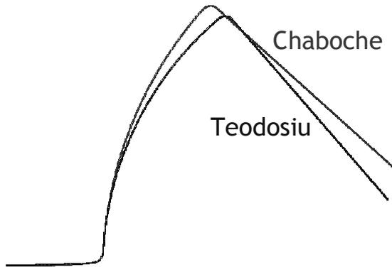
**FIGURE 3.** Springback predictions for a strip drawing test with smaller tool radii, using combined isotropic-kinematic hardening models.
