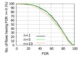
Fig. 4: CCDF of the end-to-end PDR in function of the maximum no. of bottlenecks advertised (n)
