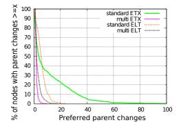
Fig. 7: Stability of the DODAG when using ELT and ETX in standard/multipath
