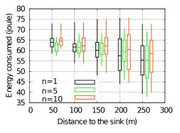
Fig. 5: Energy consumption of the nodes in function of their physical distance from the sink
