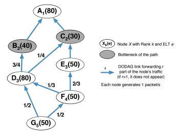
Fig. 1: Path selection with ELT (MinHopRankIncrease=1)
